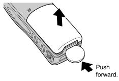
Replace the battery. Then place the battery leads inside the groove, otherwise the leads may be damaged when closing the cover.
