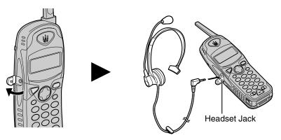
When the optional headset is connected to the handset, make sure to use the headset to talk with the caller. If you want to have a normal cordless phone conversation, disconnect the headset.
