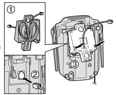
4 Connect the telephone line cord. Mount the unit, then slide down.
